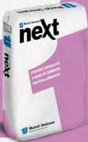
**Buzzi Unicem Next** identifies a family of hydraulic binders based on calcium sulpho aluminate clinker obtained by the burning of a mix of bauxite, gypsum and limestone at a temperature of approximately 1,350°C subsequently ground.
